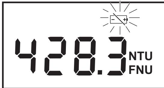
The batteries are nearly empty and should soon be exchanged. The instrument still measures with the specified accuracy.
