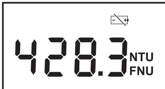
In this case, change the batteries immediately. The instrument might no longer measure with the specified accuracy. If the batteries are too weak to measure, the turbidimeter switches itself off. It can only be switched on again when the batteries have been replaced.
